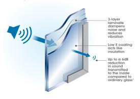
Viridian has engineered ComfortHush™ to reduce unwanted noise entering homes and buildings, whilst providing improved energy efficiency performance. ComfortHush™ 6.5mm and 6.88mm provides a 6dB improvement compared to
