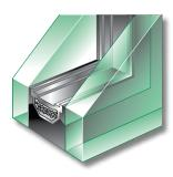
ThermoTech comprises two panels of glass separated by a metal spacer that is sealed with a primary vapour and a secondary seal to provide a hermetically sealed airspace. The spacer has a desiccant to prevent moisture forming inside the ThermoTech unit.
